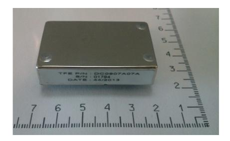
From 28 Vdc aircraft network, the converter aims to provide 18 V and 5 V outputs to supply internal integrated control panel subassemblies.
