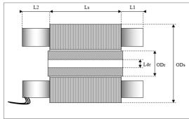
Outside dia. Stator (ODs) Outside dia. Rotor (ODr) Stack lamination length (Ls) End turns length (L1) End turns length wires output side (L2) Inside dia. Rotor (Ldr)
