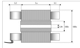
Outside dia. Stator (ODs) Outside dia. Rotor (ODr) Stack lamination length (Ls) End turns length (L1) End turns length wires output side (L2) Inside dia. Rotor (Ldr)
